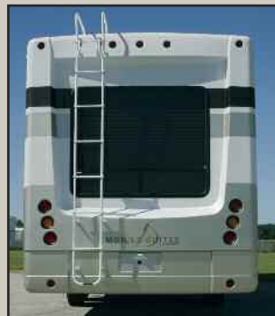
Automotive L.E.D. stop, turn, tail and clearance lights for reliability, greater visibility and safety.
