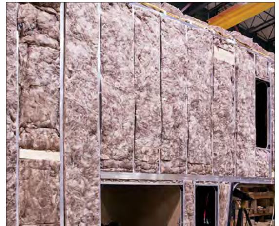
The coach and slide outs have aluminum wall studs and roof trusses positioned 16" on-centers, and the aluminum sub-floor joists are 14" on-center. Residential style high density wool insulation, in the side walls, is glued into place to prevent future settling. All spaces and voids are filled with wool insulation as well.
