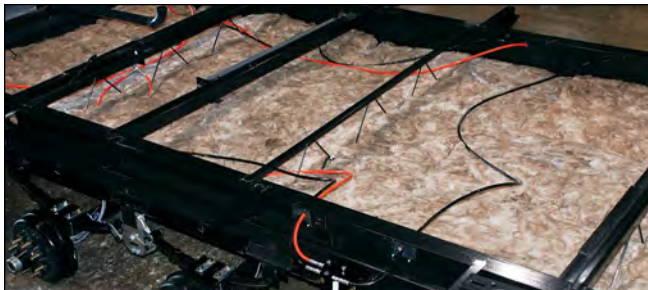
All aluminum sills and wall studs are mechanically joined and the aluminum sill tubing is fully reinforced internally with wood, providing greater strength and stability when it is "bolted-through", never screwed, to the sub-floor structure and the steel frame below.
