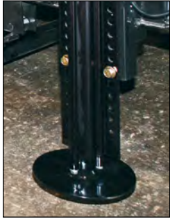
Standard Level-Up™ provides maximum stability with six heavy duty hydraulic jacks.
