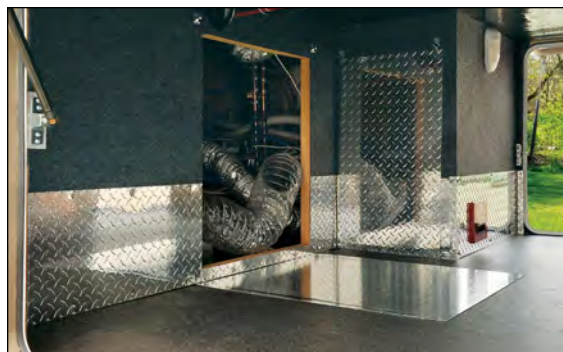
The large pass-through basement storage area is felt lined and provides abundant space for extended travel lifestyles. The copper water manifold system is easily accessible and heavy duty basement doors open easily and close securely with two gas assist lift arms and lockable slam latches.
