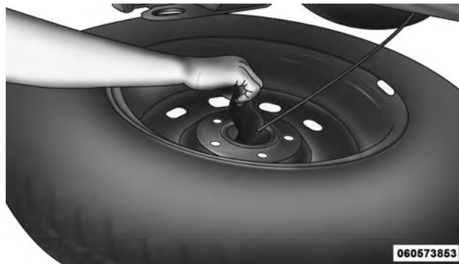
Reinstalling The Retainer
