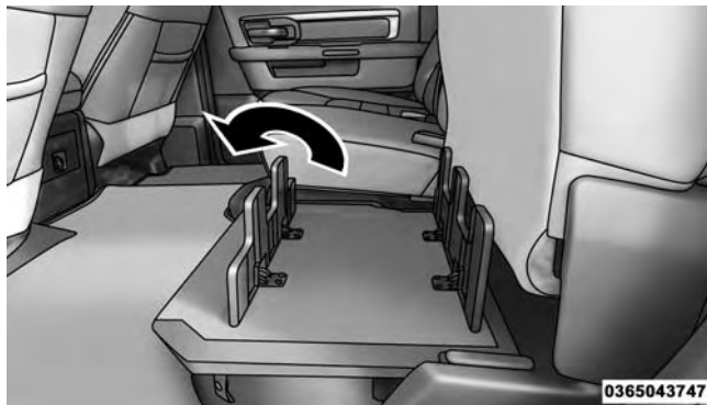
Load Floor Legs In Opened Position
