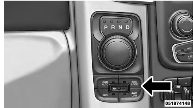
Transfer Case Switch (Five-Position)
