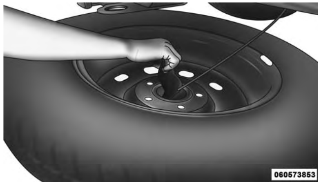
Reinstalling The Retainer
