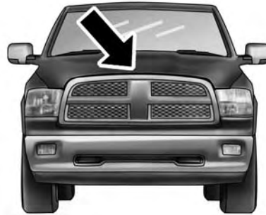
Safety Latch Location (1500 Series Shown)
