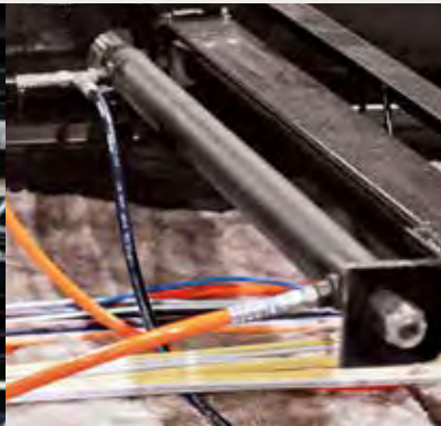
Commercial hydraulic rack & pinion slide-outs. All gear boxes are located inside the frame for the ultimate weather protection.
