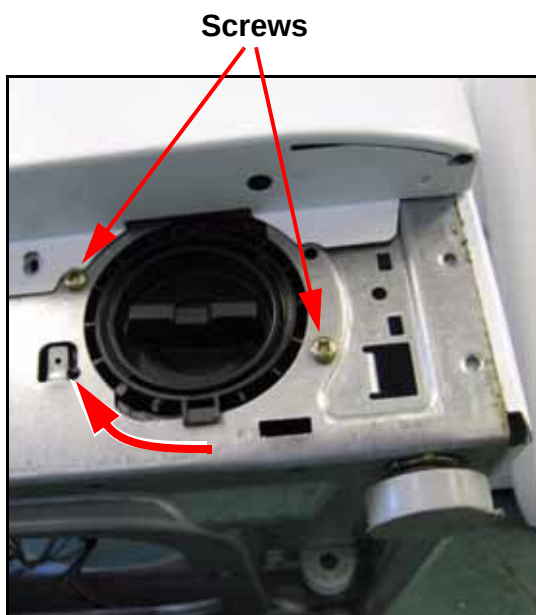
Fig. A Remove screws & rotate clockwise
