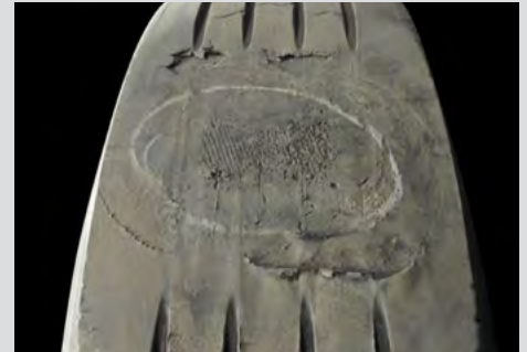
Brake Skid Damage
