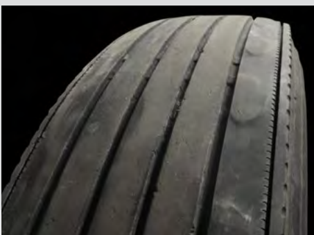
Depression Wear (Shoulder)
